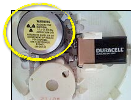
Typical Ionization Smoke Alarm Showing AM241 radioactive warning sticker
